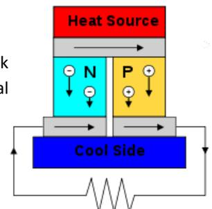
Figure 11: Schematic representation of a Seebeck generator
