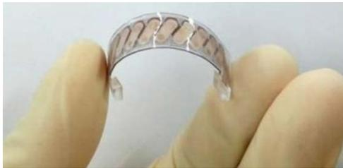
**Figure 14: thermoelectric generator**
