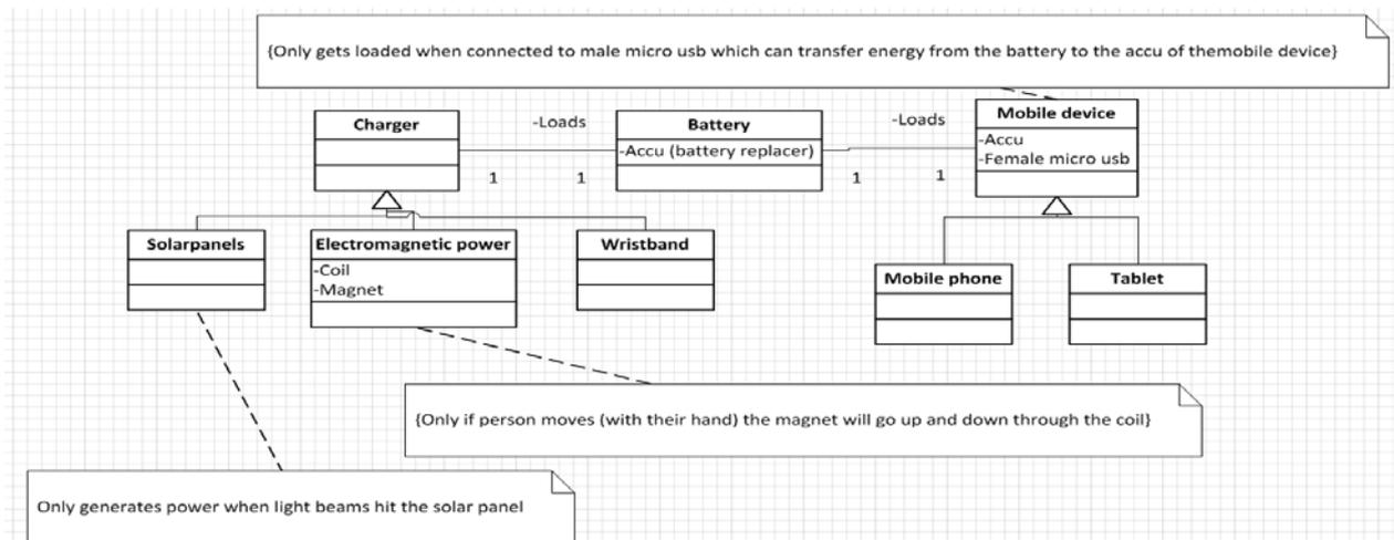
Figure 2: Block definition diagram of how the Enycharge charges a mobile device
