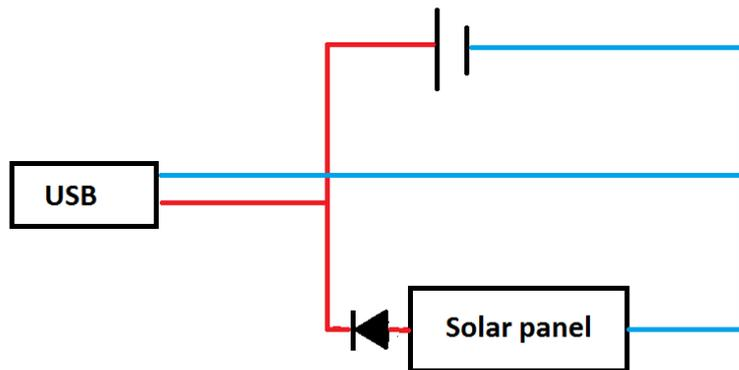
Figure 10: Circuit of the connection of the solar panel and USB to the battery
