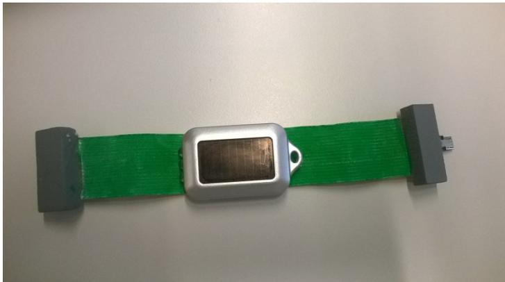
**Figure 6a: Picture of the prototype of the Enycharge**
