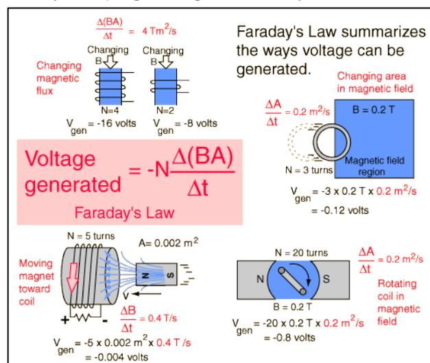
**Figure 15: Explanation of the coil-magnet system**
