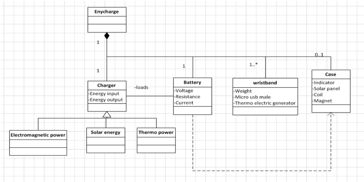
Figure 1: Block definition diagram of the Enycharge
