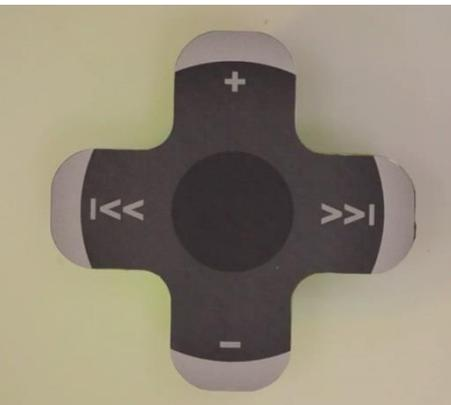
The shape of the device also creates an inherent feedback when used, when a side of the device is pushed to use a certain functionality the weight of the device makes the user feel that the device wants to return to its previous state. By returning to its initial position the devices shows that the action has occurred and that a new action is possible.
